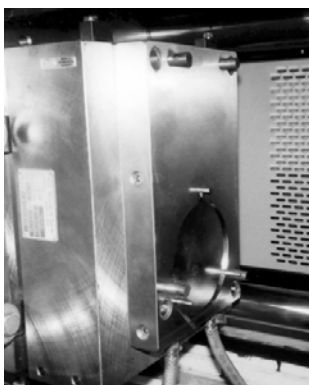
Figure 6.2-5: Shielding Disk Mold
