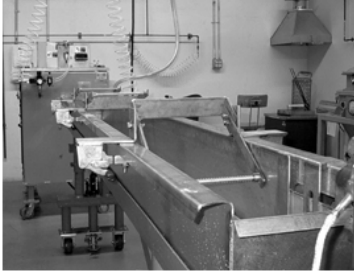
Figure 6.2-3: Pelletizer and Waterbath
